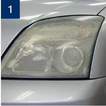
1 BEFORE Matting / yellowing, slight superficial scratches to the coating.
