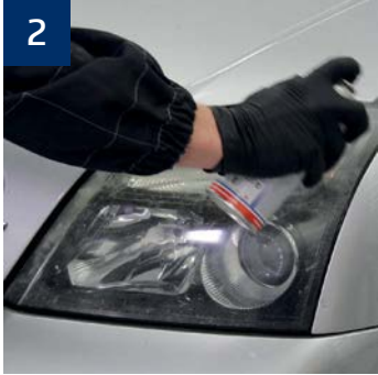
2 CLEANING Clean the entire surface of the headlight with Wax & Grease Remover 3680094 prior to masking.
