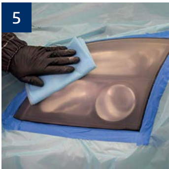
5 PRE-PAINT Clean surface with Wax & Grease Remover followed by use of tack cloth.
