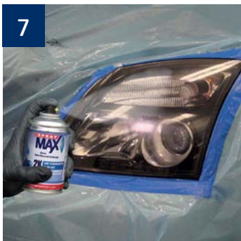
7 APPLY 2K 2 IN 1 CLEARCOAT Apply a thin even coat of 2K 2in1 Clear 3684068. Allow a flash time of 10 min at 68°F/20°C and apply a medium wet coat for film build and finish.
