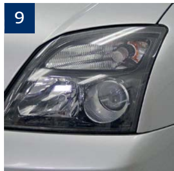
9 AFTER Once dry, surface is permanently sealed. If necessary, can be wet sanded and polished.
