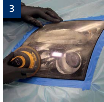
3 SANDING Sand evenly the entire surface of the headlight starting with P180 grit followed by: P320, P500, P800, P1000 and finish with P2000.
