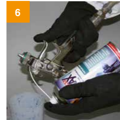
Turn the gun around and spray out any residual paint (leave air supply on minimum setting).
