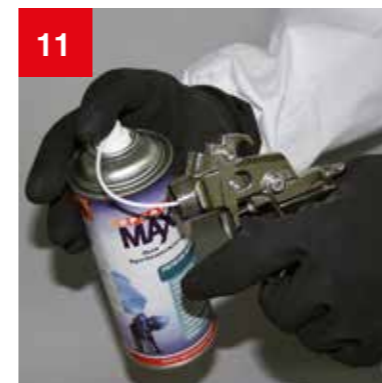
Spray out residual paint from the front.
