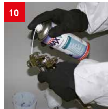
Spray out residual paint from the top (leave air supply on minimum setting).
