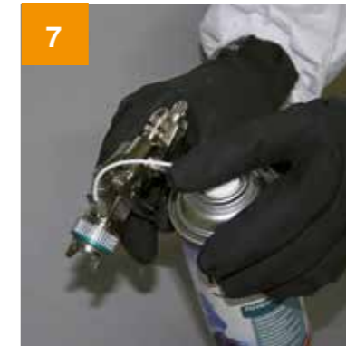
Spray out the residual paint from the top (leave air supply on minimum setting).
