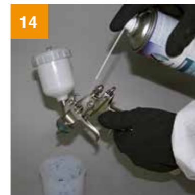
Clean the paint gun on the outside.
