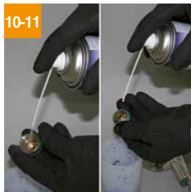
Spray off the residual paint from the front. Tilt the gun slightly downwards.
