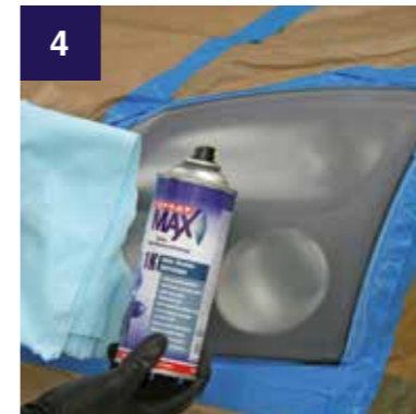
4 CLEANING Clean, remove abrasive dust with tag rag and SprayMax Aqua Silicone remover.
