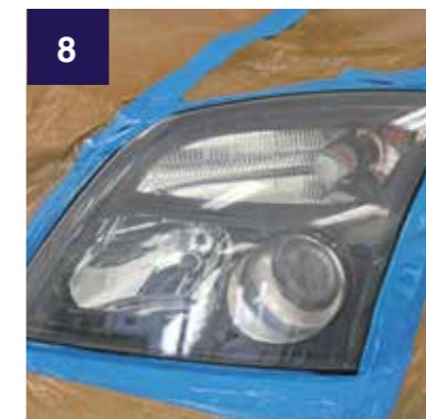
8 DRYING Drying at 20°C room temperature over night.
