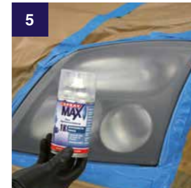
5 APPLY PRIMER Apply SprayMax Headlight Primer with one spray pass to surface until a continuous, dull film is created.
