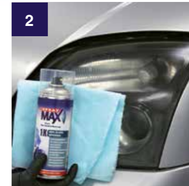
2 CLEANING Mask the rear part of the headlight and clean the surface with SprayMax Aqua Silicone remover.
