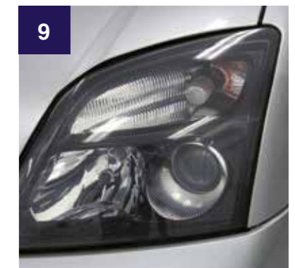
9 AFTER Headlight lens is clear. Matting, yellowing is gone.
