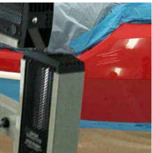
Damage: Scratched bumper. Use of an IR Lamp in between coats will aid in flash off (especially in high humidity conditions).
