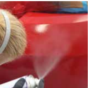
Apply SprayMax UV Spot Blender 3680091 as required through the transition area and allow to flash approximately 1-2 min. prior to curing with lamp.
