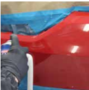
Wash with soap and water then clean surface generously with SprayMax Wax & Grease Remover 3680094.
