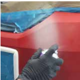
Clean surface with SprayMax Wax & Grease Remover 3680094, wipe with tack cloth.
