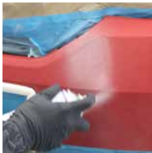
Shake SprayMax UV Primer 3680024 for 2 min. then apply 1-2 coats. Allow a minimum of 1 min. flash time between each coat of product.
