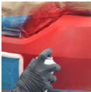
Tack surface prior to applying 1-2 coats of SprayMax UV Clear 3680059 allowing a minimum of 1 min. flash time between coats
