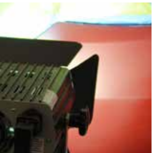
Cure SprayMax UV Primer 3680024 for 2-4 mins. depending on curing equipment (see TDS for details).
