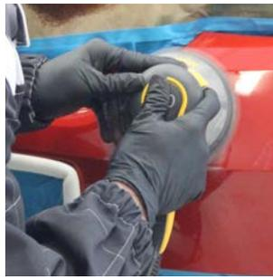
Sand damaged area using P320. Clean with SprayMax Surface Prep 3680094 then apply SprayMax Adhesion Promoter 3680009
