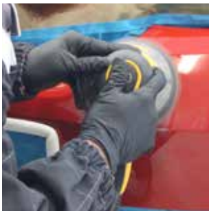
Sand damaged area using P320. Clean with SprayMax Wax & Grease Remover 3680094 then apply SprayMax Adhesion Promoter 3680009
