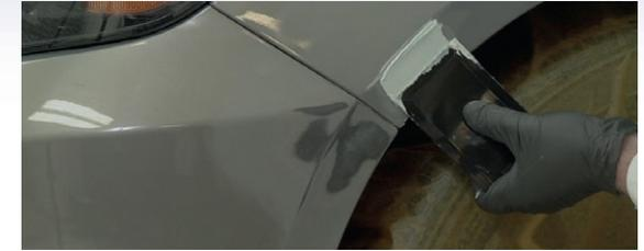
5. Apply an All-In-One Premium Body Filler to damage area and when cured, block sand with P120
