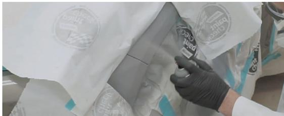
7. Mask remainder of repair area and wipe down with a dust-free tack cloth
