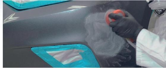
3. Mechanically sand the damaged area beginning with P120 grit abrasive then P240
