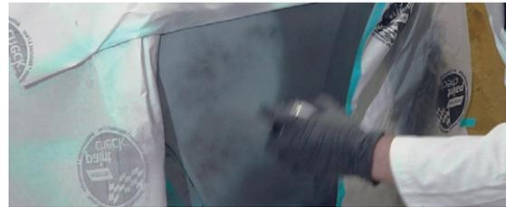
9. With IR-Heating: Distance 16 inches at 800 Watt / dry for 20 minutes – alternatively a heat gun can be used to speed up the process
