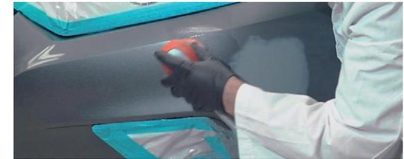
12. Clean surface with **Wax and Grease Remover 368-0094**
