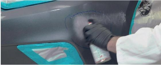
1. Vehicle is hand washed and dried, thoroughly inspected, then damaged area is compounded to remove any remaining road film and contaminants
