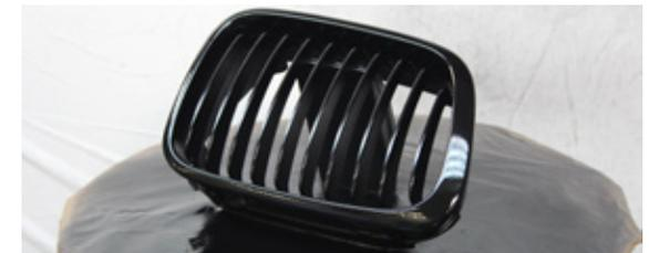
9. Let the Clear coat dry for 12h at 68°F/20°C or force dry (IR) for 15min.
