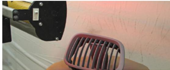
5. Dry 2K rapid Primer Filler for one hour at 68°F/20°C or force dry (IR) for 15min.
