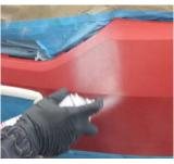
Shake SprayMax UV Primer 5680019 for 2 min. then apply 1-2 coats. Allow a minimum of 1 min. flash time between each coat of product.
