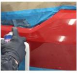
Wash with soap and water then clean surface generously with SprayMax Wax & Grease Remover 3680094.
