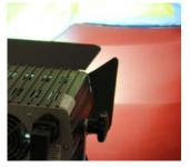
Cure SprayMax UV Primer 3680019 for 2-4 mins. depending on curing equipment (see TDS for details).
