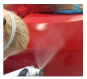
Apply SprayMax UV Spot Blender 3680091 as required through the transition area and allow to flash approximately 1 min. prior to curing with lamp.
