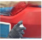
Tack surface prior to applying 1-2 coats of SprayMax UV Clear 3680059 allowing a minimum of 1 min. flash time between coats.
