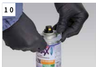
10 Fit the spray head and adapter ring to hold the cap
