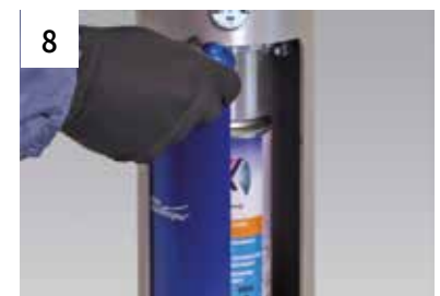
8 Close the door to the right to trigger the filling process
