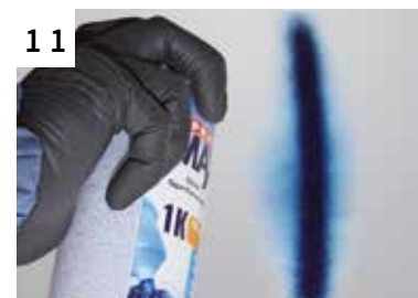
11 1. Shake the can 2. Check the colour 3. Spray the valve until empty (if necessary see TMB)
