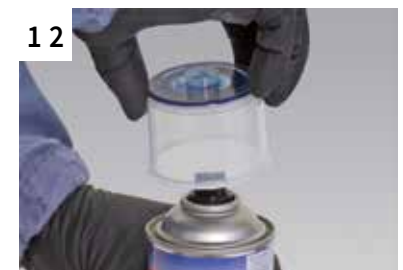
12 The pad remains in the cap to generate the colour code
