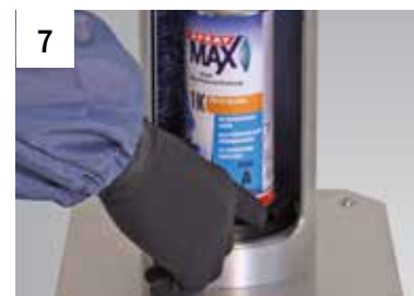
7 Turn the rotating plate of the device slightly upwards to fix the can into position
