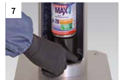
7 2K 250ml: Filling adapter is required to compensate the height during filling
