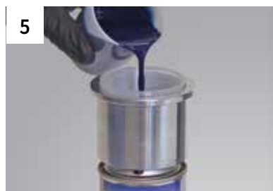
5 Fill with the mixed original paint
