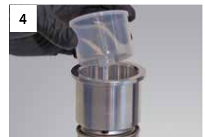
4 Place the cylinder on top, insert the FillClean cap and press down firmly
