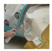
**Apply first coat** adjust variator, perform a test spray, apply
