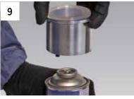
Open the door once filling process has stopped. Take can from machine and remove cylinder and cap.
