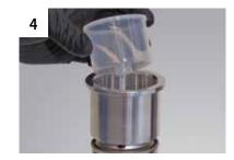
Place the cylinder on top, insert the FillClean cap and press down firmly.
