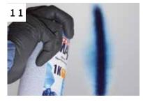
1. Shake the aerosol can 2. Check the color 3. Invert can and press nozzle to clean the valve
