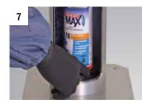
Turn the rotating plate of the device slightly upwards to fix the can into position.
