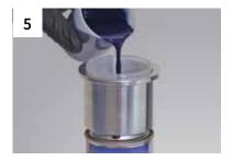
Fill with the mixed original paint. Don't pass the safety line.
