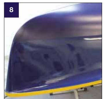
8 Repair/Paintprocess above and below water line is finished
