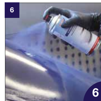
6 Apply 1K Bottompaint in 2-3 spray passes, flash off time 5-10 min in between
