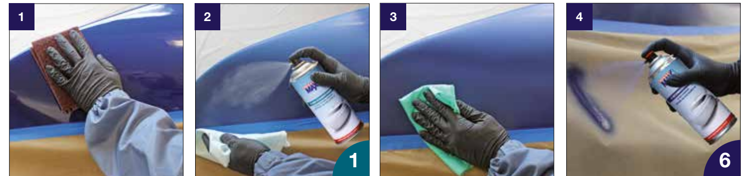
1 If necessary mask area below water line and sand with abrasive fleece
